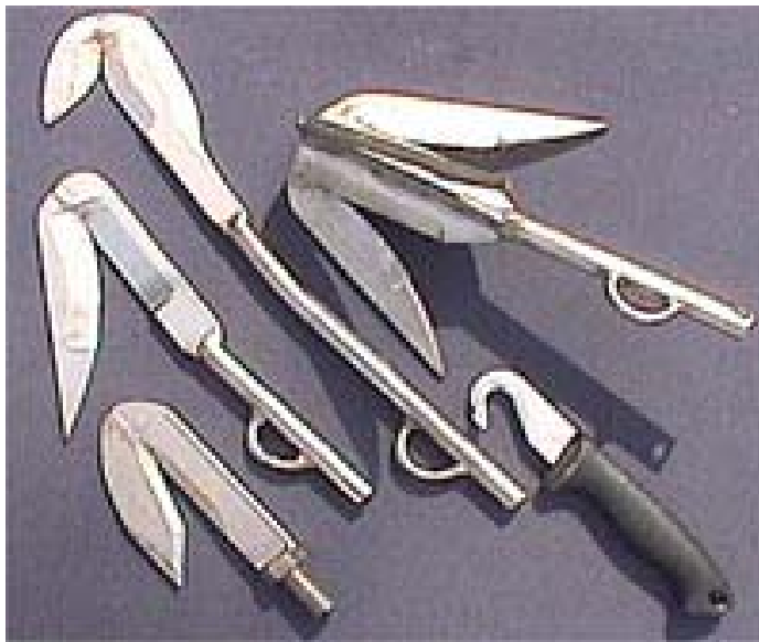
Figure 3. Knives and other cutting tools used in disentanglement. Photo: Center for Coastal Studies.
